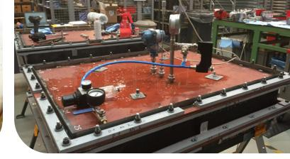
The synthetic rubber EPDM 400G had to withstand a radiation exposure of 65 rad for half an hour – and significantly exceeded this requirement.
